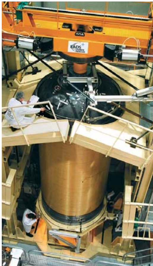
Pressure test on a missile stage in wound carbon fibre. Solid propulsion for missiles or space launchers is one of the flagship applications of nanostructured composites.
